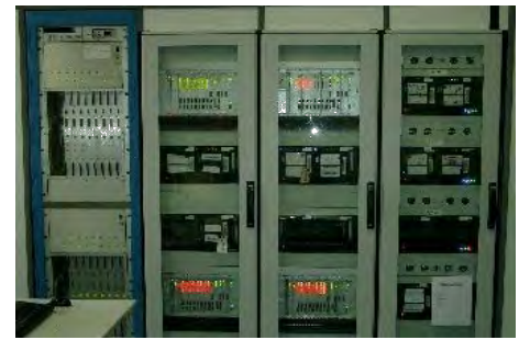
VLBI correlation unit hosted by the Max Planck Institute for Radio Astronomy
