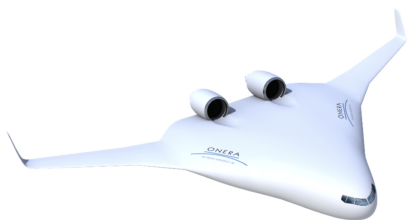
Small-Medium range Integrated Light and Efficient (SMILE) blended wing body configuration
